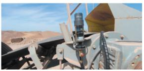
Industry: mining Application: electric motor bearings Lubrication system: NTN-SNR DRIVE BOOSTER Installation solution: remote beam clamp mount
